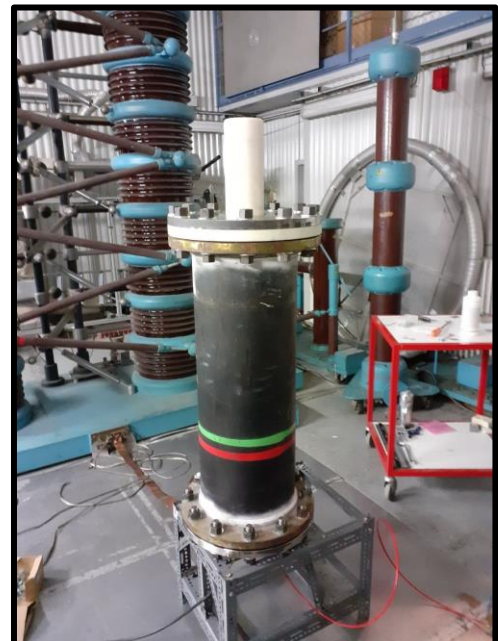
Marx generator, experimental setup
